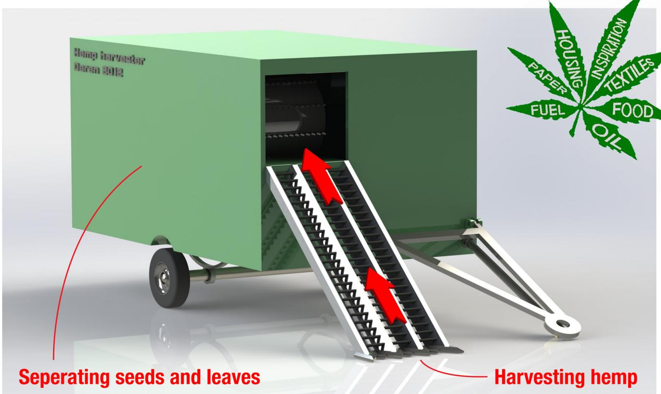
Hemp harvester is a first multifunction machine of this type in the world. It harvests the hemp, splits the seeds and leaves and connects stem into bales. Machine is constructed as a mobile unit and is easily transported to different locations. For transport a personal vehicle is required. In the machine 4 phases of plant processing are included that save us time, money and energy.
